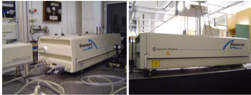
Slika 4. 21 Tsunami laser (model 3955)
