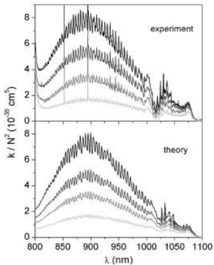
FIG. 12. The comparison of simulated and measured reduced absorption coefficients in the Rb<sub>2</sub> X-A band for four different temperatures given in Fig. 5. Quantum mechanical simulations were performed with *R*-dependent spin-orbit coupling and taking into account the weighted sum of different isotopomer contributions.
