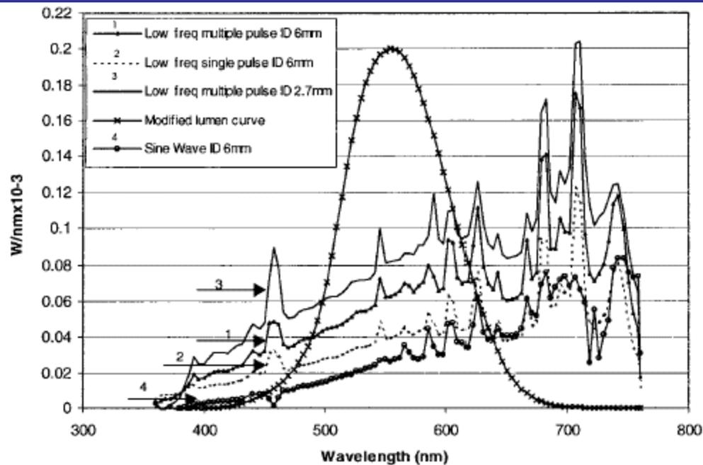
Figure 15. Spectral power distributions for the Cs lamp operated on various power sources.
